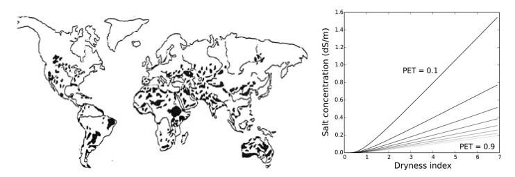
Figure 6. (left) Global distribution of salt affected soils (adapted from Szabolcs [1989]). (right) The steady state concentration of salt as defined in equation (8) plotted against the climatic dryness index D (or the ratio of potential evapotranspiration to rainfall). Each line corresponds to changes in the potential evapotranspiration (in mm/d) varying from low (dark lines) to high (light lines), while mean rainfall depth is kept constant at  $\alpha = 10 \text{ mm/d}$ .
