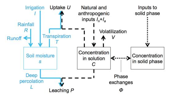
**Figure 4.** Schematic illustration of mass balances of soil moisture, s, and a generic soil compound in solution with concentration C=m /( $nZ_rs$ ) (e.g., nitrate, the soluble fraction of a contaminant, and dissolved salts). Solid lines represent fluxes of water, dashed lines fluxes of dissolved m, and dotted lines fluxes exchanged with adsorbed phase. Equations (4) and (5) describe mathematically this coupled system, forced by natural stochastic rainfall and anthropogenic inputs.
